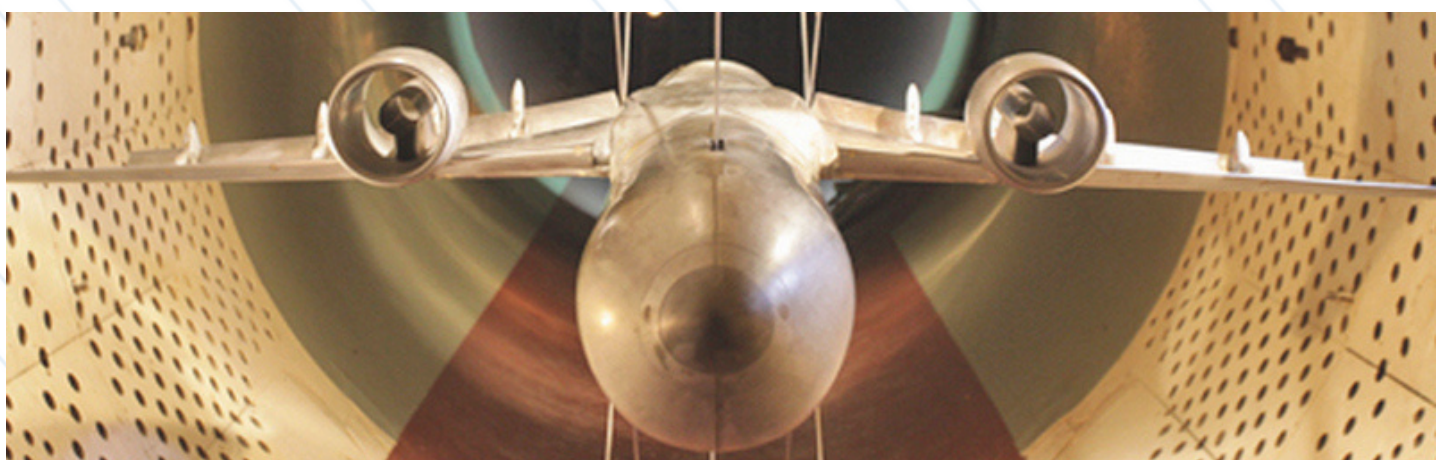
Installed Engine Noise Attenuation (IENA), joint cooperation project in the field of aeroacoustics, TsAGI (Russia), the Aerodynamic Research Institute AVIC (ARI, China), the Federal University of Santa Catarina (UFSC, Brazil), BRICS Framework Programme 2019
